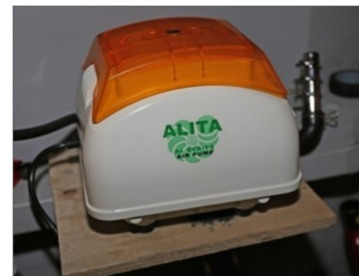
Luftpump 40 l/minuten, 48 Watt
