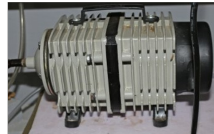
Kompressorpump 125 l/minuten, 136 Watt
